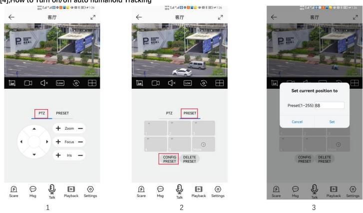
1,Control the PTZ button to rotate the camera to your desired position (set a Return position)
